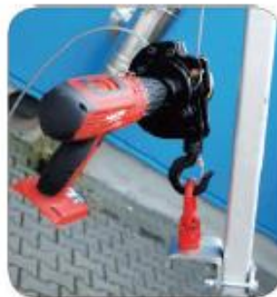
Fixed at the tripod, using an adapter plat with stop ring
