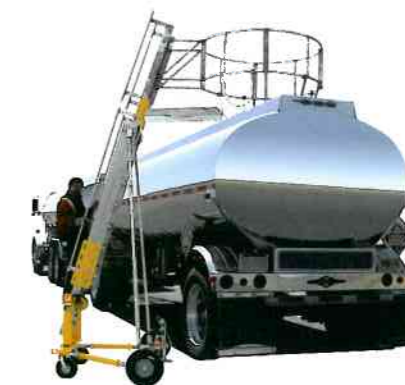
Ladder shown with Pneumatic Wheel Kit, 26"-42" (660 mm - 1067 mm) Step-Out Platform, 16" (406 mm) Fall-Out Bar Assembly and the 5.5ft (1.52 m) Diameter Guard rail Cage.
